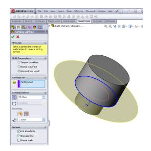
4. Add Tooling Split\*Mold Tools.Insert Sketch, and then set block size.
