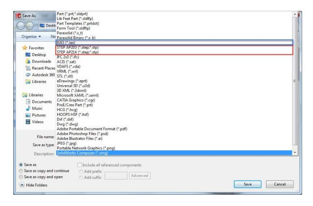
First design your model in solidwork and save it as Step or IGES format
