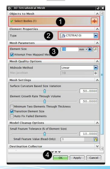
In this step mesh will apply to geometry.
