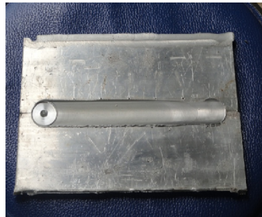
Figure (2-3).Two 6063-T4 Al-alloy plates to be welded before and after FSW.
