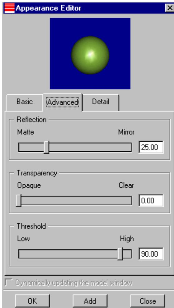
The Advanced tab controls how the lights are reflected off of the object. The Reflection slider controls how the room will be reflected in the rendered image. Unfortunately, this shininess can't be seen until the object is rendered so take the default value for now (this functionality is improved in Revision 21 of Pro/E). The transparency slider works great for windows, cut away views, etc.
