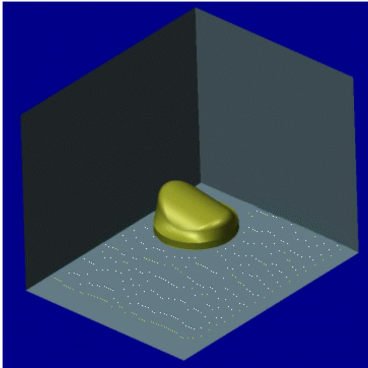
The size of the room is somewhat subjective. Its size should be such that it is larger than the part but still be somewhat square so that the wall textures are not distorted when the image is created. Orient the part to a nice isometric view and zoom in close enough so that the edges of the room cannot be seen. Make the room larger or smaller if necessary. You may also need to adjust the light locations.
