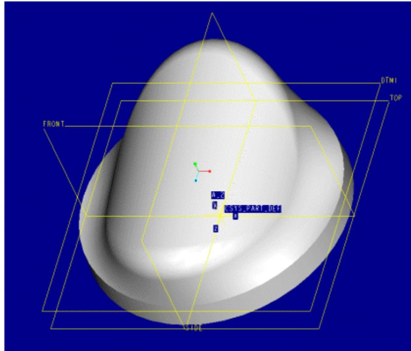
Before we begin we need to make sure we have saved a front or side view of the part. This will be used later to easily place the object on the floor of the room. Next, turn off all the datums, curves, spin center, etc. They won't be needed to create the image. Now the colors and appearances need to be defined and added to the object. This is found under View-Model Setup.
