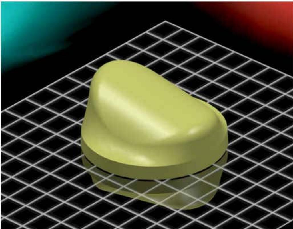
This is the result of our first effort. To make the image more realistic, perspective can be used. Pick the Perspective button. This will distort the room and part, but will make the image look much more realistic. Adjust the amount of perspective by using the Eye Distance slider (see below). Don't use too much perspective or the result will look too distorted!
