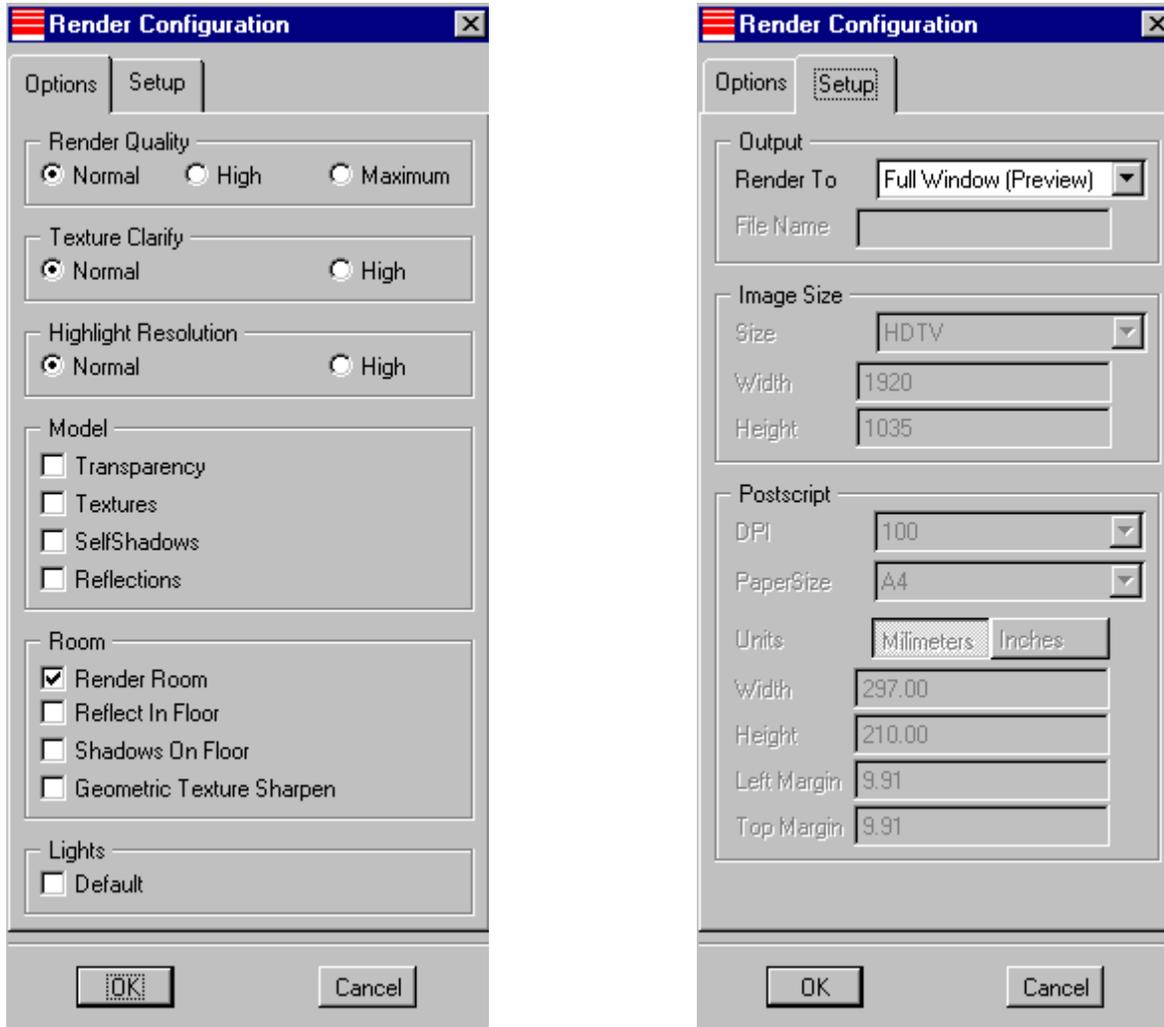
Some of the best looking renderings occur when only the part is rendered, the room is only reflected in the part. Make sure the default lights option is unchecked; lights have already been set up.
