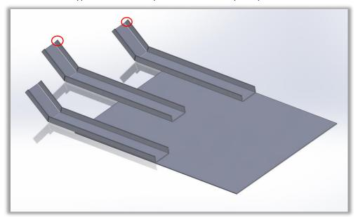
2. Suppose you want to add a pipe below these two edges as shown above and in the middle of the flange. To do that draw two lines on the flange like below. Use the flange surface to draw the lines:
