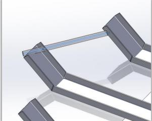
7. This is after mating. You may have to move the pipe to make pass through both flanges.
