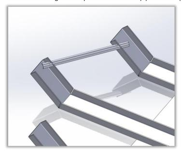
8. Now the pipe is passing through the flanges and you need to cut it. Select the face in the assembly to draw a sketch
