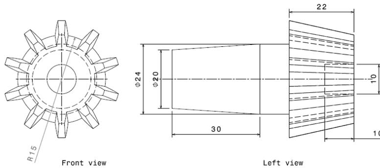
9. Larger Bevel Gear (Define same gear teeth profile as that of Smaller gear teeth)
