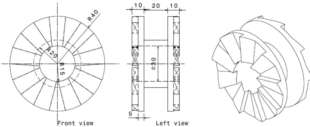
11. End Clutch (Staggered Teeth Clutch: Design same teeth profile as that of Clutch 1)
