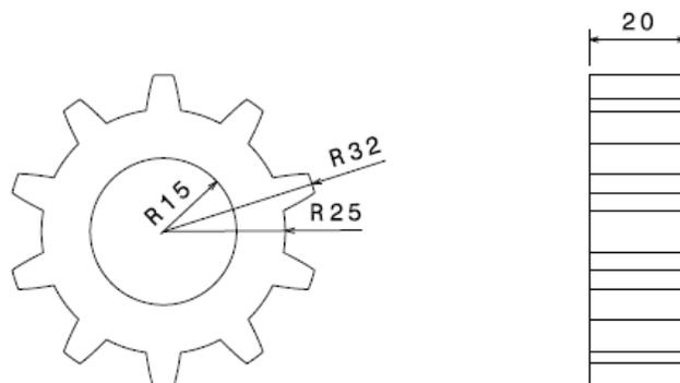
14. Larger Spur Gear (Define same gear teeth profile as that of Smaller Spur gear teeth)
