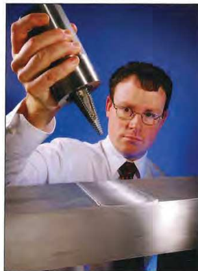
Above left This aluminium butt joint profile is being made using friction stir welding.
