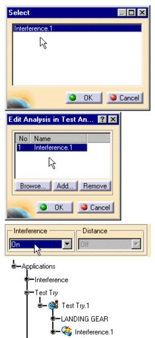
10. To locate the clash position more precisely, set the Interference combo to Stop in the Edit Simulation dialog box
