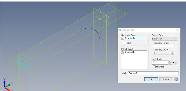
I have made the cross section of pipe based around a standard 50NB heavy pipe. This sweep becomes the configuration "bent"
