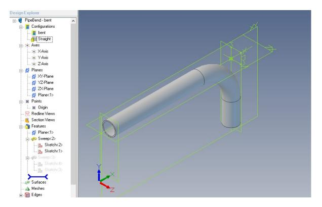
I have used Alibre Design here but the same basic method will work with Solid Works, Solid Edge and Inventor. I have modelled a section of a bend in a pipe and made two different configurations. This is the configuration I have named bent.
