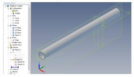
This configuration I have named straight. By switching between the different configurations I can display the pipe bent or straight.
