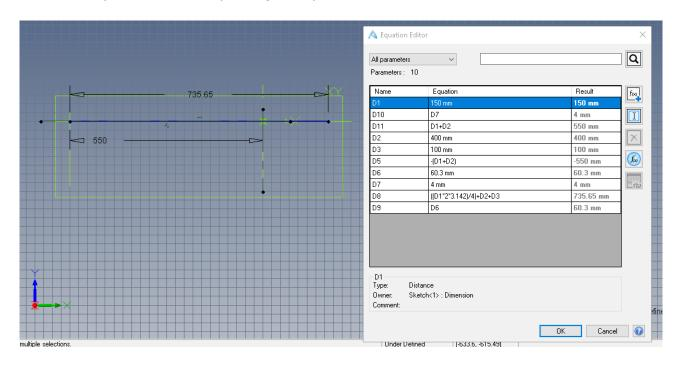
The total length of the line I have used for the sweep path has been calculated from the dimensions used in the sketch used in making the path for the bent version of the pipe. This is the formula in D8:
