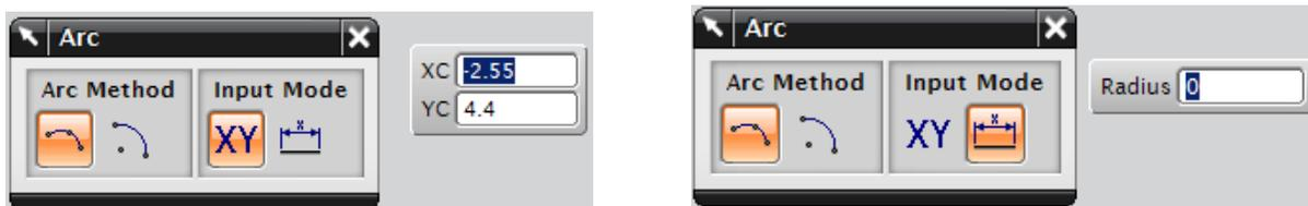
The second option creates the arc with a center point, radius and sweep angle or by center point with a start point and end point. The illustration is shown below:
