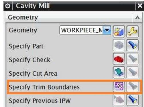
The **Trim Boundary** window will pop up. Make sure to carry out the following procedure in the right sequence. Keep the default setting of **TRIM SIDE** to **INSIDE**. This tells the software that the cutter should not cut material anywhere inside the boundary. Trim allows you to specify boundaries that will further constrain the cut regions at each cut level.
