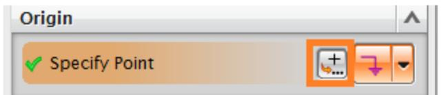
The **Point Constructor** box will open. The **XC**, **YC**, **ZC** points should have a default value of 0.
