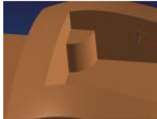
Add edge blends at the corners as shown in the final Model below. Keep the value of blend as 10 radii for outer edges and 5mm radii for the inner edges.
