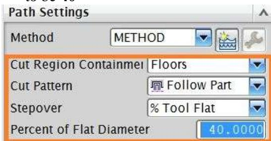
In flooring operations, it is always better to keep the Stepover value to be less than half of the diameter of the cutter in order to achieve more flatness on the planar surfaces.
