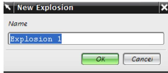
Now the UG environment is in *Exploded view* environment though you do not find any difference. When we start exploding some assembly, we should decide upon a component to keep that component as the reference. This component should not be moved from its original position. In the case of the impeller assembly, the impeller will be the right option as it is central to the entire assembly. Now let's start exploding the components.
