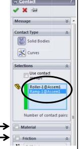
We will add friction later, but our initial simulation will be easier to verify without friction. In the Elastic Properties section, note that the default is set as "Impact," with several other properties (stiffness, exponent, etc.) specified. At each time step, the program will check for interference between the
