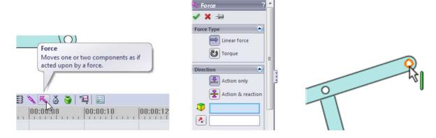
The direction box is now highlighted. Rotate and zoom in so that you can select the top face of the Frame part. The force will be applied normal to this force. As you can see, the force acts upwards.
