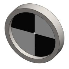
Note that the mass of this part (40.14 lb) is almost identical to that of the other wheel, but the mass moment of inertia (837.0 lb·in²) is about 37% greater. The mass moment of the part depends not only on the part's mass, but also on how that mass is distributed. As more mass is placed at a greater distance away from the axis of the part, then the mass moment of inertia about that axis increases (note the  $r^2$  in the equation for I on page 1).
