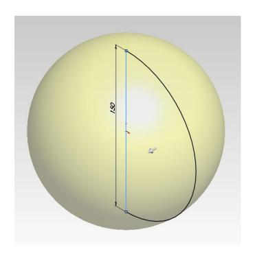
Now we have ready our model to add a text (you can try wrap feature if you want, to confirm that it doesn't work on spherical faces). After we model our sphere, we click on front plane and we click on reference geometry -> plane and we create an offset plane, out of the sphere. (this step is optional, as i've done it in order to see in what direction the split line is going in the next step).
