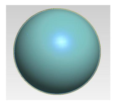
After that, we go to our feature tree -> solid bodies -> Revolve and click hide. This is done because in the next step we're going to create the text and split line it on the offset surface. We don't want to click on the body's surface because it will not
