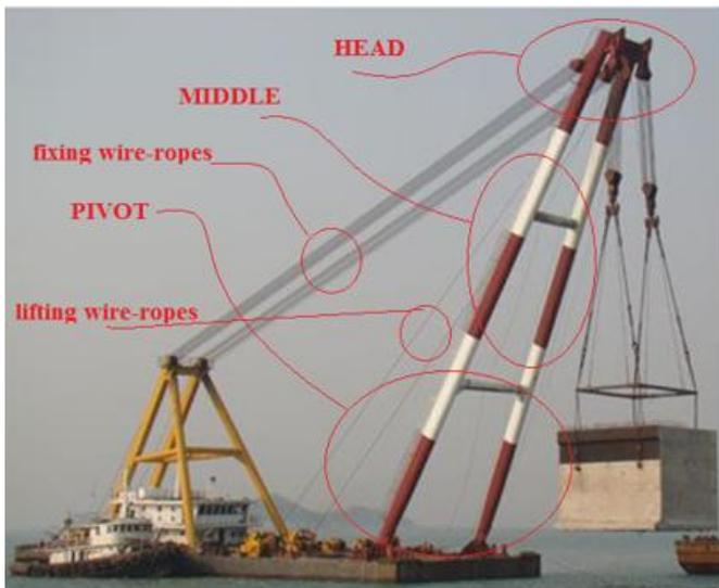
Fig -4: Sheerleg crane, type Welded box girder legs
