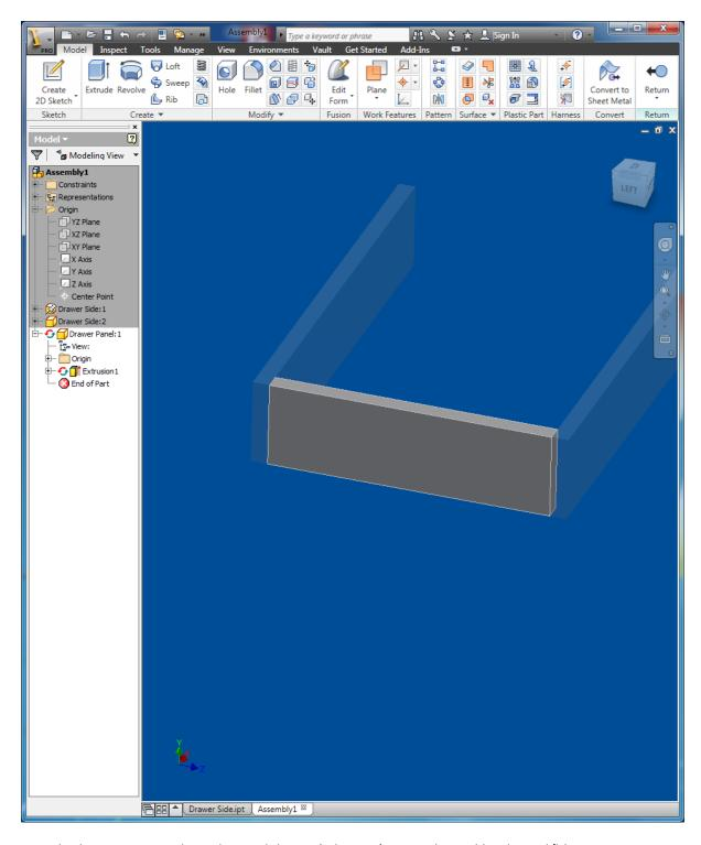
Extrude the part. Notice how the model is an 'adaptive' part indicated by the red/blue arrow icon
