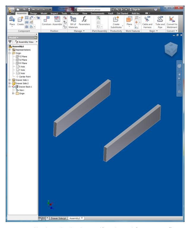
Create an assembly with two sides. Aligned to top and front edges, inside faces use a mate offset
