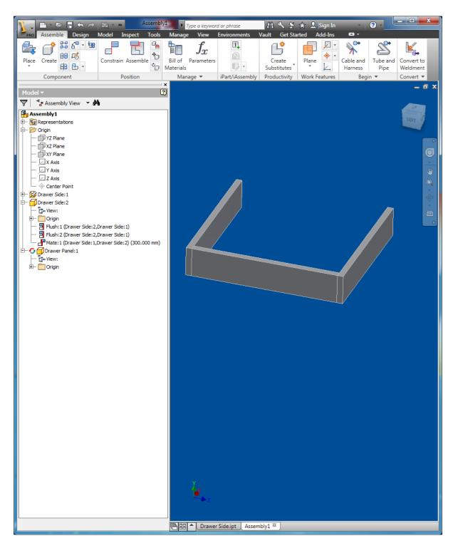
Finish the part by pressing the return button. Drawer width as shown 300mm
