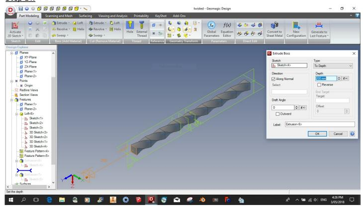
To complete the part I require, I am adding straight section to each end. this is a simple extruded profile.
