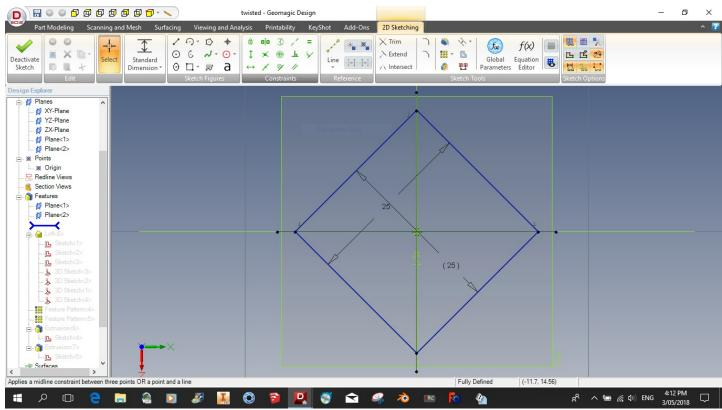
A sketch is now made on the middle plane. again this is for a 25  $\times$  25 square, but as this is on the mid point of the twist, the sketch is rotated 45 deg.
