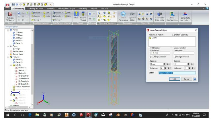
As , in this case I wished to have features symmetrical to base plane, I patterned twists each side of this plane.
