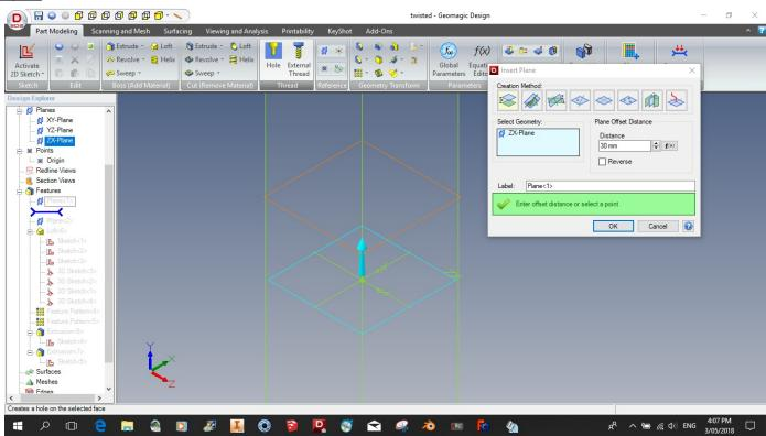
A new plane is constructed, in this case 30mm from the base plane. As the length of one twist is to be 60mm this plane needs to be 1/2 the twist pitch Step 2.
