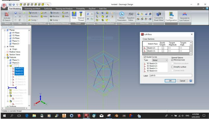
We now loft the 3 profiles to produce a section of twist. The 3D sketched are used as guide curves to control the loft
