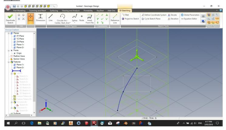
Step 8 continues the process of linking the corners of the profiles with a 3D sketch.
