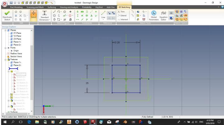
A sketch is now made on the base plane. As, in this case the twisted section is to be 25 x 25 square the sketch is dimension as above. I is important that this sketch is symmetrical to model origin.
