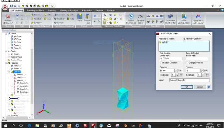
The feature pattern tool is now used to make the number of twists required.
