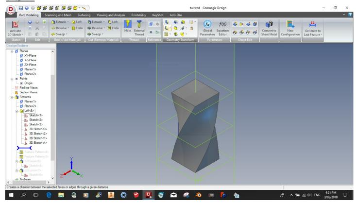
The completed loft forms 1 pitch of twisted section.
