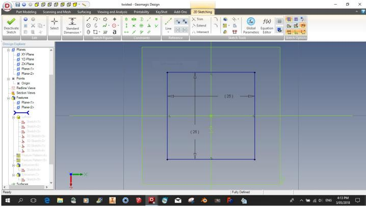
The final sketch is now made on the 3rd plane. again this is for a 25  $\times$  25 square, This sketch is made symmetrical with the sketch on the base plane.
