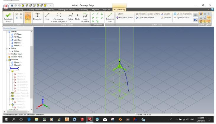
A 3D sketch is now made. This sketch connects the corners of the three profile corners as shown above.
