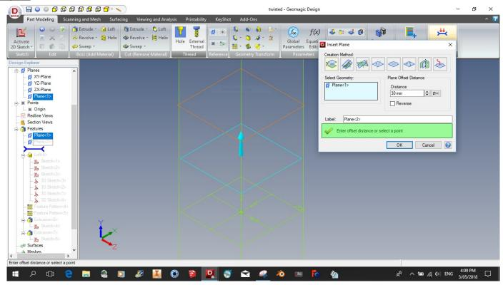
A second plane is constructed 30mm from the first constructed plane. This plane is positioned from the first plate 30mm as this is half the first pitch.
