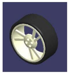
Notice how the wheel rim changes based on the family table match while the tire model is simply flexed based on the values given it. This is also evident in the model tree -- TIRE.PRT stays the same, but WHEEL.PRT becomes either RIM1 or RIM2.
