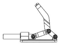
2. Click Alternate Position View on the Drawing toolbar, or click Insert, Drawing View, Alternate Position.
