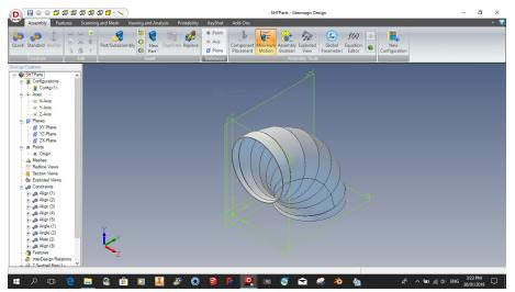
On the left is the completed 7 segment bend. I started detailing these types of bends before CAD, then with the first 2D CAD software and now with 3D modeling software. The method I use is made up from my knowledge of producing developed patterns using these three aproaches.
