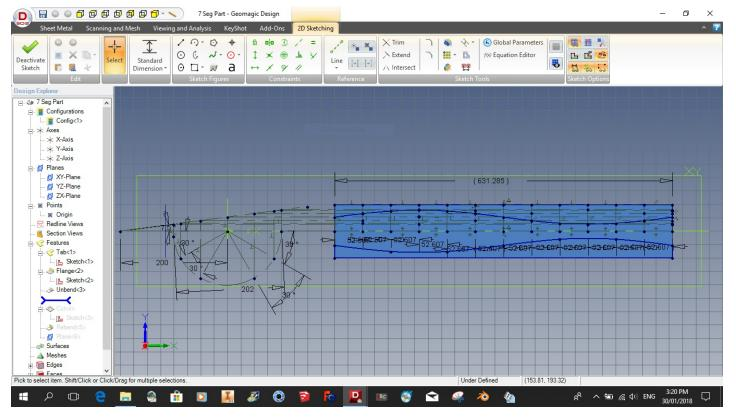
The full patern segments are produced the same way. The sketch used to cut the sine curve can be mirrored to produce both sides. Though I have not tried it, the required sine curve could be generated in a spreadsheet, then used to drive the cut sketch.
