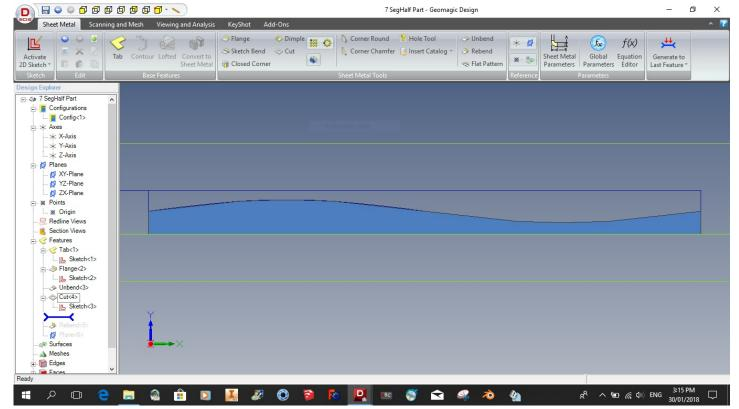
And now we have completed flat pattern. We can then roll back into modeled sheetmetal part with the flat pattern for generating CNC files to cut on profile cutting machines.
