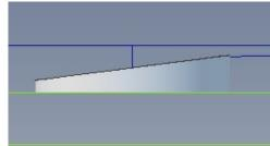
As with all standard lobsterback bends, the start and finish segments are basically a normal segment cut in half. The location of the segment seam, see image of finished bend, assists the fabricator in lining up the parts to assemble the bend.
