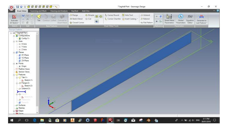
Next we flatten this cylinder, and a sketch is places onto the plane of the flattend cylinder.
