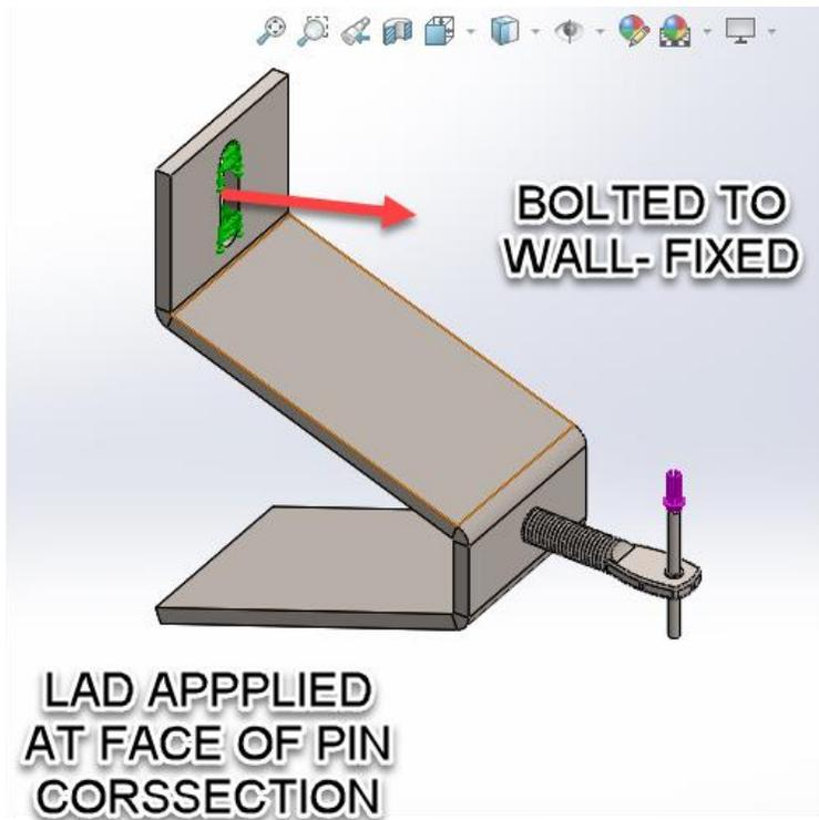
To perform a stress analysis , I used fixed geometry at the slot region and applied the load on the pin which is con nected to the marble .
