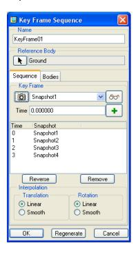
You can double click on each of them to see their corresponding snapshot. Now, we want a effect such that all it 'fly out' parts, and later 'fly in' to form the original assembly. To do this, we need have the following sequence: Snapshot1, Snapshot2, Snapshot3, Snapshot3, Snapshot3, Snapshot2, Snapshot1. So, you can get this by select the snapshot from the dropdown menu:
