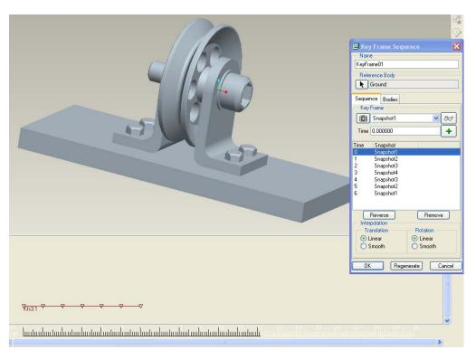
Click on "OK" to close the 'Key Frame Sequence' window. Now, you can drag each snapshot to the appropriate timeline location, to design how long you want each snapshot transfer to another. An example is shown:
