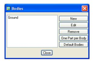
This is where you define ground part and moving part (the default is all part is grounded). We can quickly define all parts are moving parts by selecting "One Part per Body'. Once you do this, notice all the parts now have a reference frame of their own.
