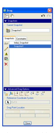
Make sure you expand the 'Snapshots' menu and the 'Advanced Drag Options' menu. Now, you can either select the part you want to move from within this window, or you can select it directly from the model window, we will use the later one. Now, we want to move all four of the screws in the z-direction. So select the 'Advanced Drag Options' menu, and use your mouse to drag the pin to appropriate location:
