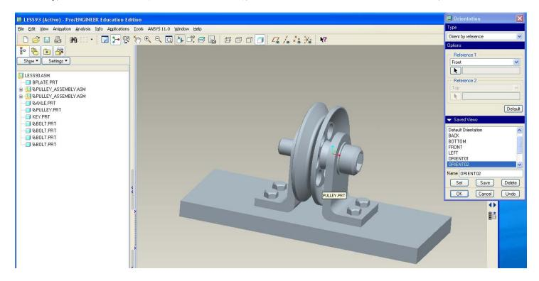
Now, the final orientation we want is rotate the part about 180 degree, and save this orientation as "ORIENTO3":
