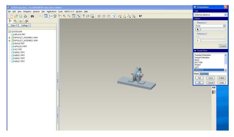
This is the first orientation we want. Now create a second orientation that have a close look at the pulley assembly, use the zoom out (middle mouse scroll), then save this orientation as "ORIENTO2", as shown below:
