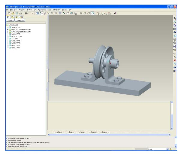
To create a new keyframe sequence (snapshots), we need to first define the ground and moving parts. Click on the (Body definition in animation) button, the following menu will pop up.
