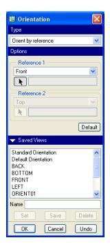
Create the first 'orientation': move the pulley assembly further away (zoom out), and name this orientation as "ORIENTO1", click 'save' button to save this orientation:
